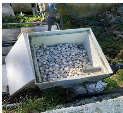
Figure 4: Geopolymer in cylinder format
