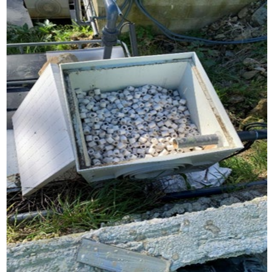
Geopolymer cylindric form in a sump (125)
